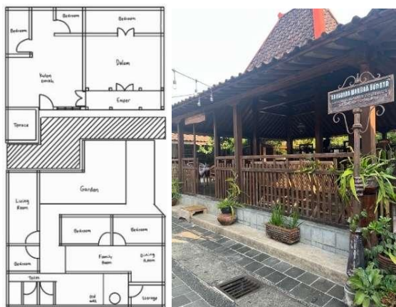
Figure 5. Traditional housing layout with the ndalem facing the pendopo . The pendopo in Gang Rukunan RW 09 is used as a shared space.
