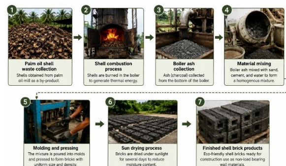
Figure 1. Shell Brick Production Workflow
