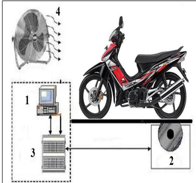
**Figure 1. Dynamometer test scheme: (1) monitor, (2) dynamometer roller, (3) GPU (graphic processing unit), (4) high-tension cable, (5) measuring burette.**
