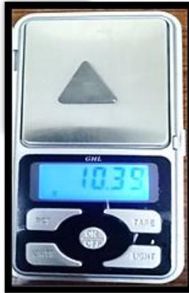
**Figure 1. Weighing the initial weight of the insert tool**
