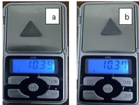
**Figure 4. Mass wear (a) before, (b) after**
