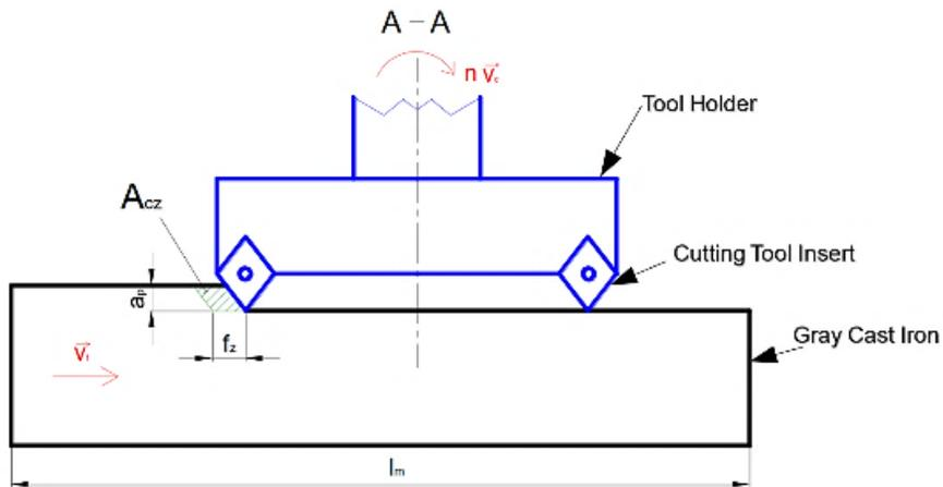
**Figure 2. Machining face milling type shoulder cutting [15]**
