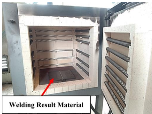
Figure 2. Furnace Machine Room
