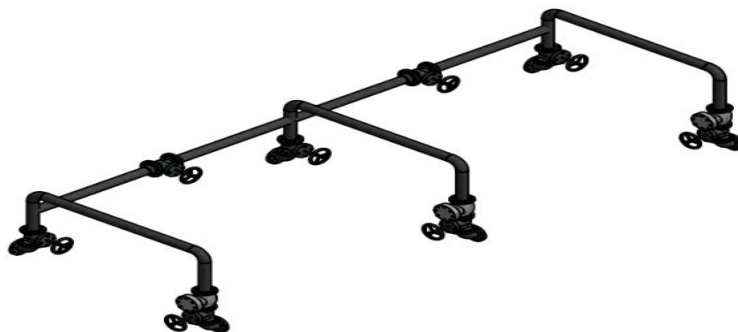
Figure 6. Modification Pipeline 3D Model Pipeline compressor
