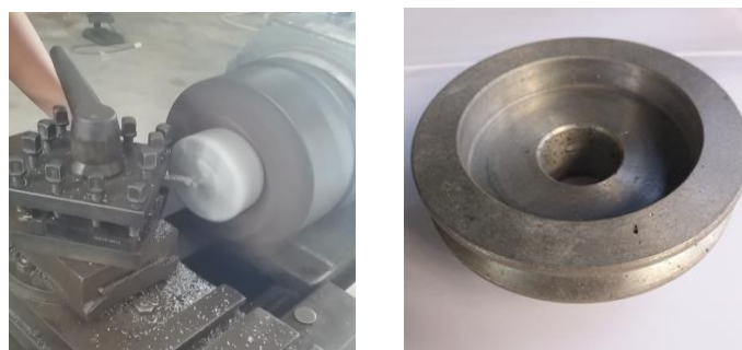
Figure 6. Machining Process of the As-cast Pulley
