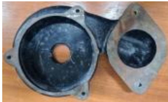
Figure 1. Condition of the pump casing before damage
