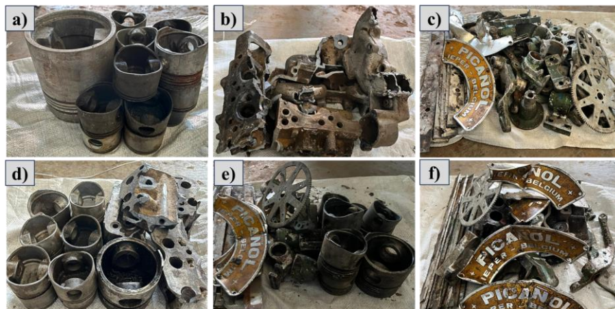
Figure 5. Aluminium waste: a) pistons, b) piston and engine blocks, c) piston and loom, d) engine blocks, e) engine block and loom, and f) loom
