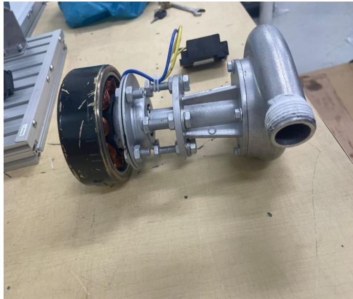
Figure 2. Picture of the francis turbine model coupled with electric generator
