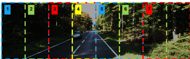
Figure 4. The image is divided into 7 regions. The width of each region is 25 percent of the image's width, and the stride is 12.5
