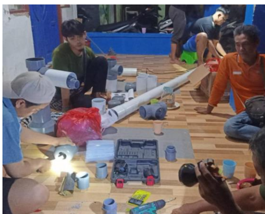
Gambar 2. Proses Pembuatan Repeated Processing Septictank (RPS)
