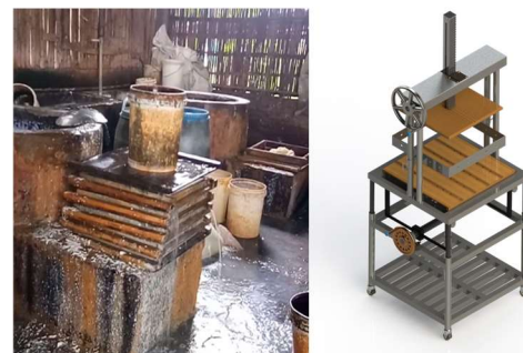
Figure 6. Comparison of design plans of printing & pressing work facilities before and after repair
