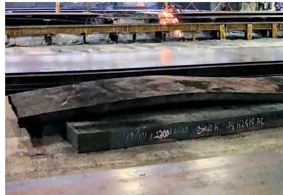
Figure 5. Wavy Edge Defect
