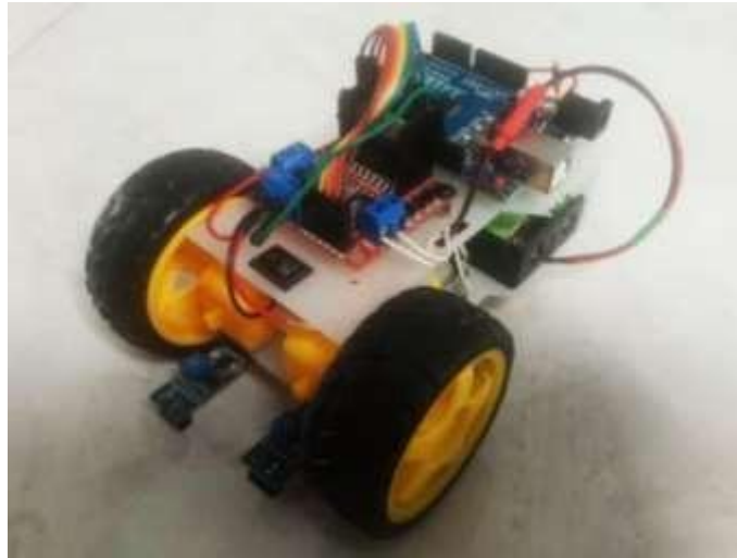
Gambar 5. Rancangan Model Robot Line Follower
