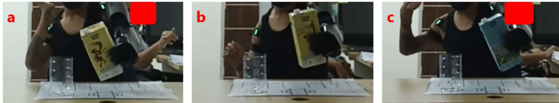
Figure 2. Three kinds of prosthesis operating mechanism during the drink box pouring task: (a) pushing the non-amputated arm forward, (b) pushing the amputated arm forward, and (c) pushing the non-amputated arm sideways
