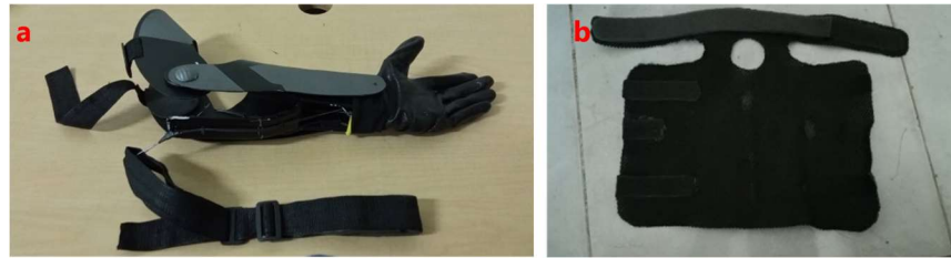
Figure 1. Appearance of the Panangan Prosthetic Hand: (a) the body of the prosthesis and (b) the socket of the prosthesis
