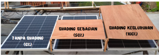
Figure 6: Solar panel shading test conditions
