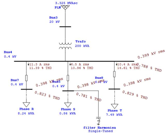
Figure 12: THD Values After Installing the Filter
