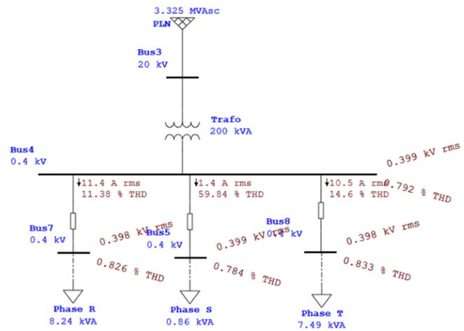
**Figure 11:** Simulation Results Before Installing Single-Tuned Filter
