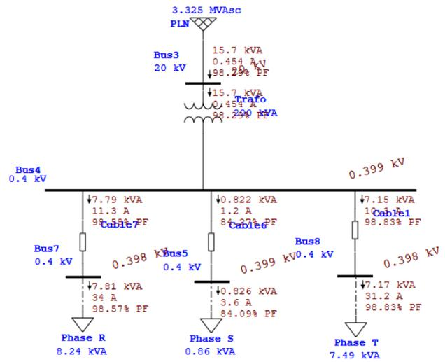
Figure 10: Load Flow Simulation Circuit
