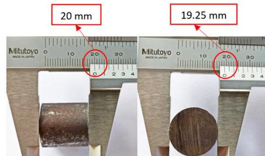
Figure 3. Sample sizing before hardening.
