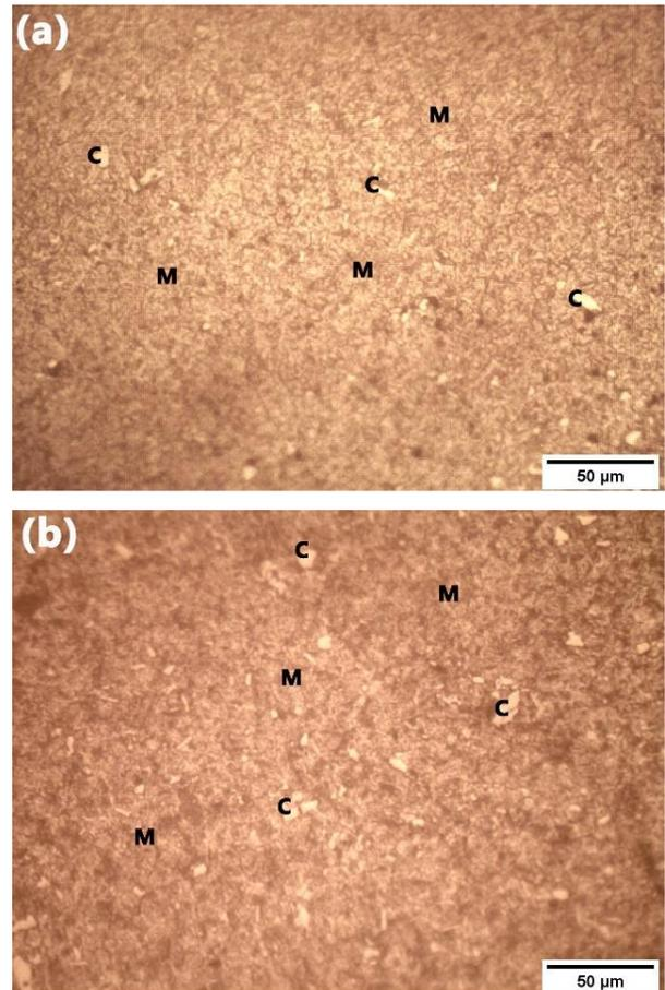
Figure 7. The SKD 11 tool steel microstructure after hardening (a) air cooling and (b) oil quench.
