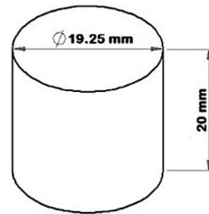
Figure 2. The size of the sample used for hardness test and microstructure observation.
