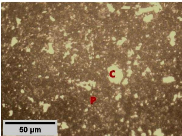
Figure 1. D2 tool steel microstructure before heat treatment (C is carbide: bright area, P is pearlite: dark area).
