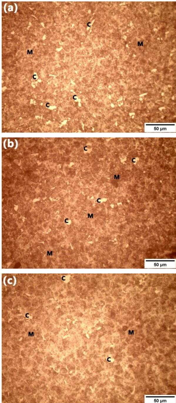
Figure 8. Microstructure of SKD 11 tool steel after tempering at 250°C, variations in holding time (a) 15, (b) 30, and (c) 45 minutes.
