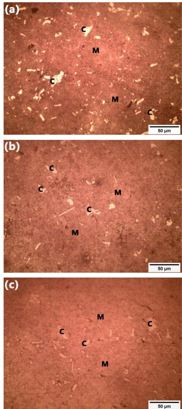
Figure 9. Microstructure of SKD 11 tool steel after tempering at 400°C, variations in holding time (a) 15, (b) 30, and (c) 45 minutes.
