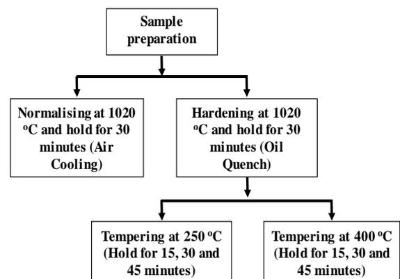
Figure 4. Heat treatment process.
