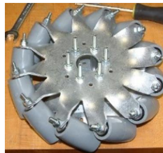
(b) Omni wheel for mecanum drive
