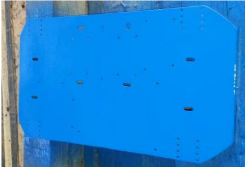
Figure 5. Base structure of MWMR prototype.
