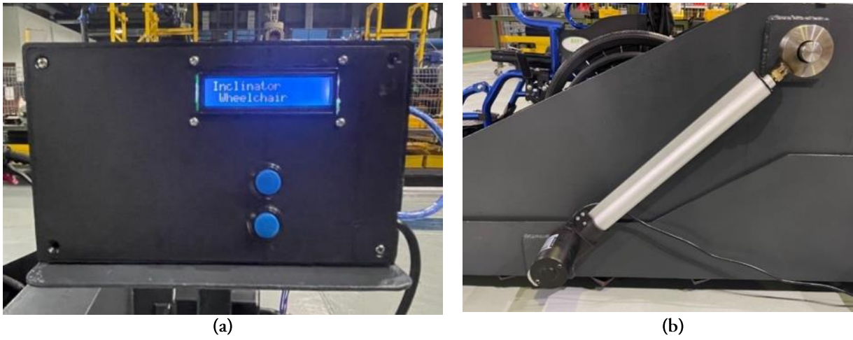
Figure 12. Liquid-crystal display (LCD) and switches for (a) the actuator and (b) the actuator for the wheelchair recliner.
