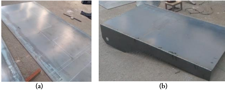
Figure 8. (a) Marking and measuring on mild steel and (b) Welding of the outer side of the wheelchair recliner.
