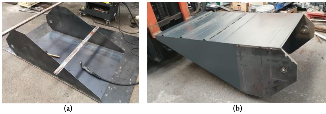
Figure 8. (a) Marking and measuring on mild steel and (b) Welding of the outer side of the wheelchair recliner.
