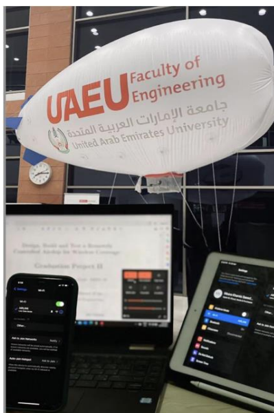
Figure 8. Indoor testing of the wireless coverage of the airship.
