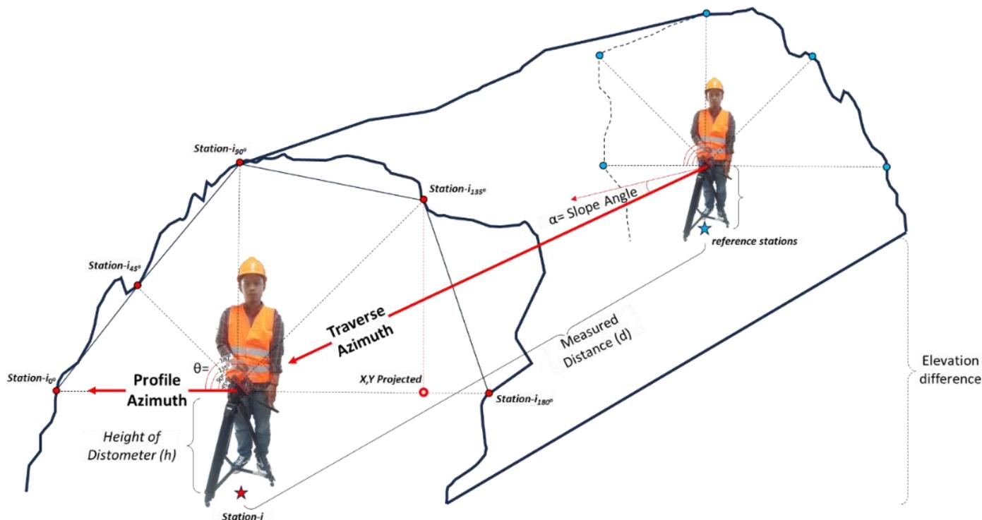
**Figure 4.** Geological Compass, Leica Distometer D510, and Tripod as primary tools were used to get a relative height of the cave’s attic, which was then transformed into a corrected position using ArcGIS 3Dsoft software.
