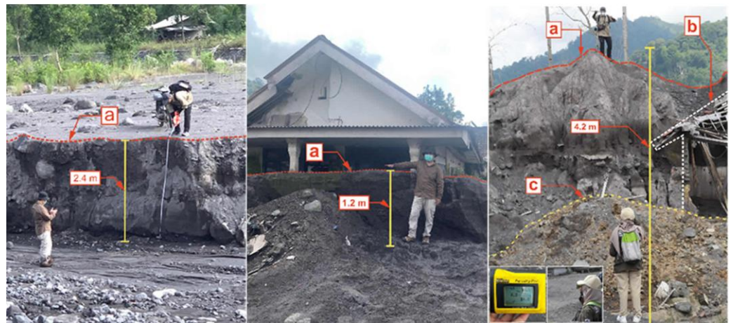
Figure 10. Field Thickness Measurement Methods. These methods include direct measurement using a tape measure (left), estimation of affected objects (center), and profiling measurements using a distometer (right). Note: (a) lahar material deposits, (b) affected buildings, (c) lahar deposition.
