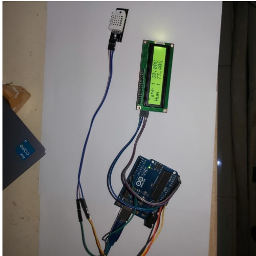
Figure 9: DHT22 Sensor Testing with LCD
