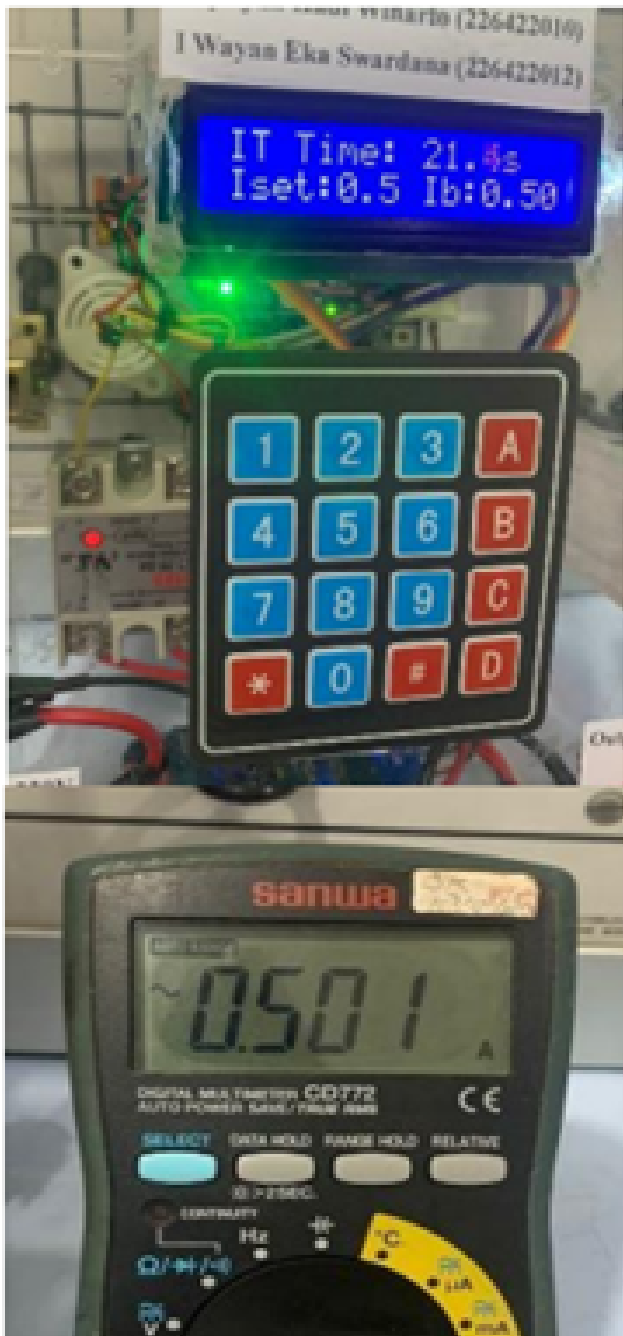
Figure 4: Solid State Relay (SSR) testing with a HIGH signal
