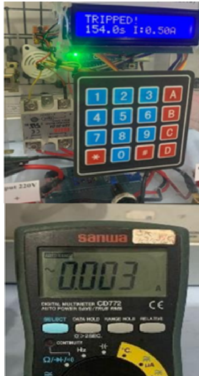
Figure 5: Solid State Relay (SSR) testing with a LOW signal
