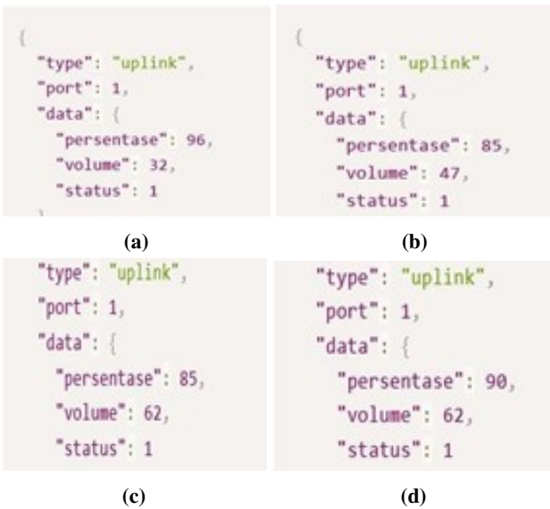
Figure 6: Data Transmission Results from LoRa to Antares (a - d) Data Sent Successfully
