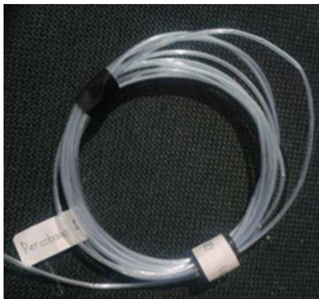
Figure 11: Filament result from recycled PET testing at various speed/temperature settings.
