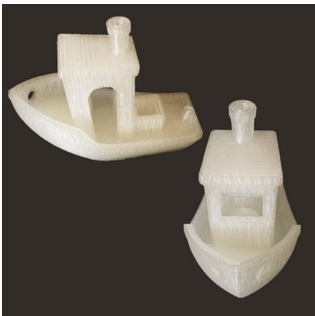
Figure 10: 3D Benchy test using PLA filament and recycled PET for comparison.
