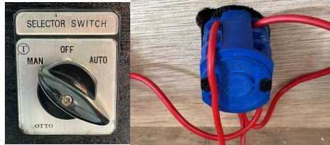
Gambar 2. Selector switch posisi manual
