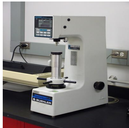
Figure 4. Buehler hardness tester, made in the USA. (The author took the photo).
