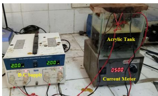
Figure 3. Actual experimental setup of monopolar parallel (MP-P) electrode.
