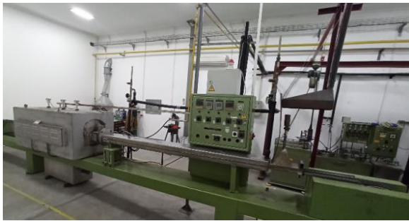
Figure 2. Heating furnace and quenching canal.
