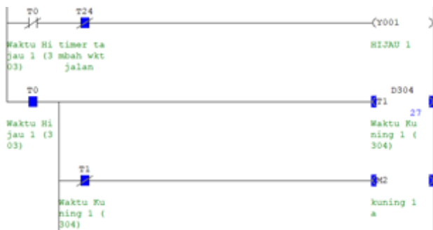
Figure 10: Ladder diagram view of yellow light at intersection 1
