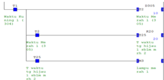
Figure 12: Ladder diagram view of red light at intersection 1
