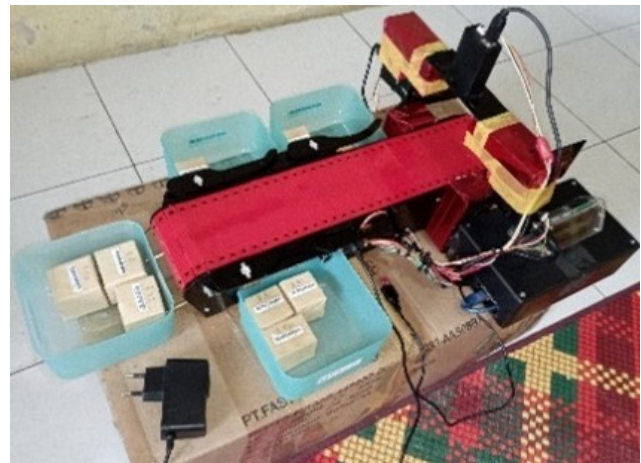
Figure 9: Hardware results of the Barcode Scanning Conveyor Automation system tool.
