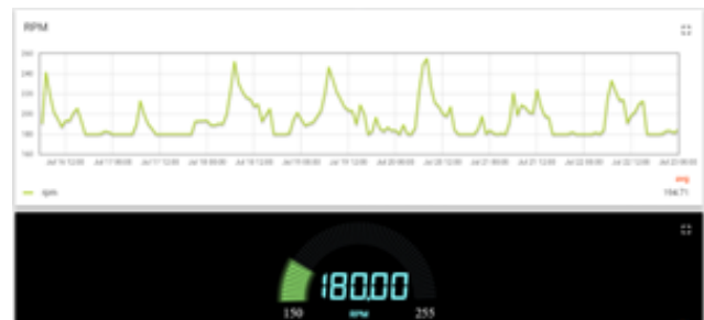
Figure 7: Fan RPM Monitoring Results based on Fuzzy system temperature and humidity inputs
