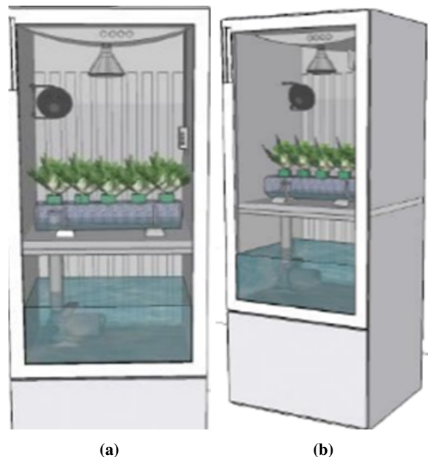
Figure 4: Smart Showcase Prototype 3D Design; (a) Front view, (b) Side view
