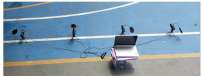
Figure 3: Data collection with microphones arranged linearly
