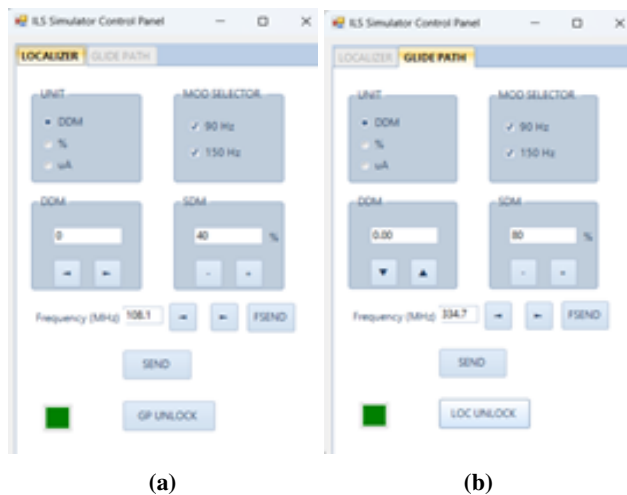
Figure 4: GUI display of the ILS Simulator design (a) Localizer (b) Glide Path
