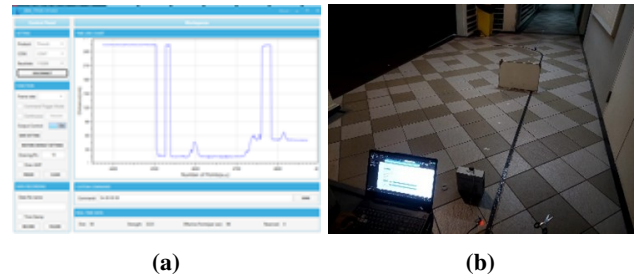
Figure 12: Proximity sensor testing using BW_TFDS software
